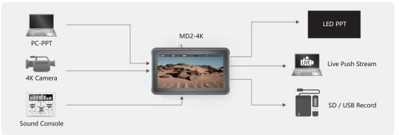
Scenario 3: Live Streaming and Recording Integrated with Video Conference (Fixed the UVC Channel as Camera View for Video Conference, While Offering Dual-camera Live Streaming and Recording)
